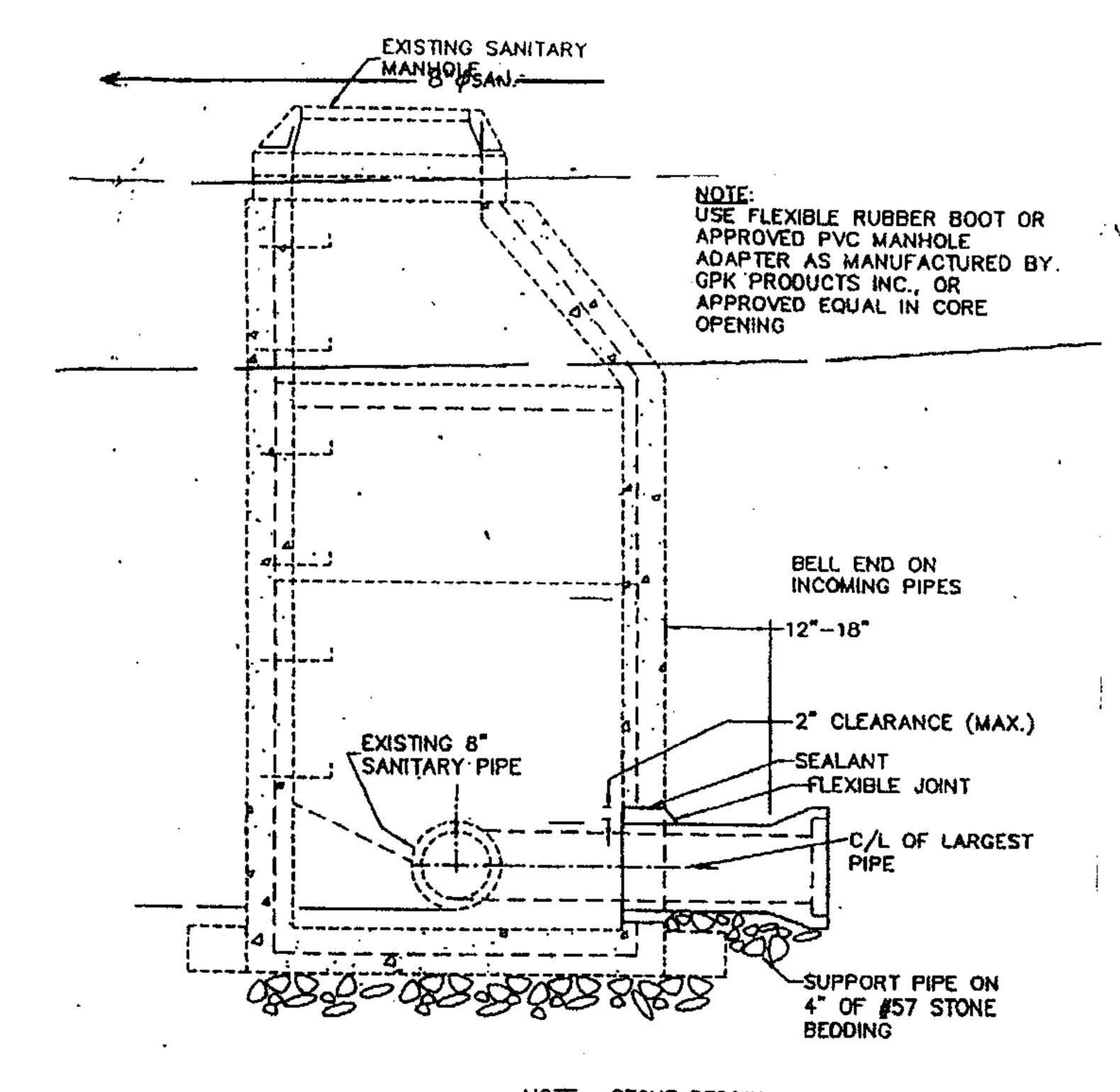
NOTE: STONE BEDDING SHALL EXTEND TO THE OUTER BOUNDARY OF ALL UNDISTURBED AREAS SURROUNDING THE MANHOLE.
