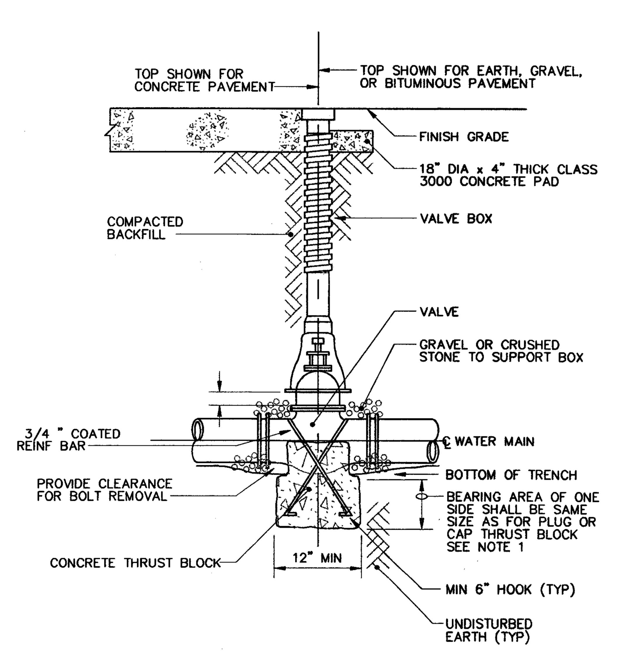
THRUST BLOCKS REQUIRED ON VALVES 12" AND LARGER DIAMETER.
