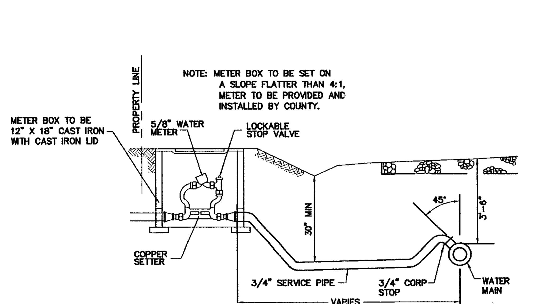
DETAIL — WATER SERVICE CONNECTION NO SCALE
