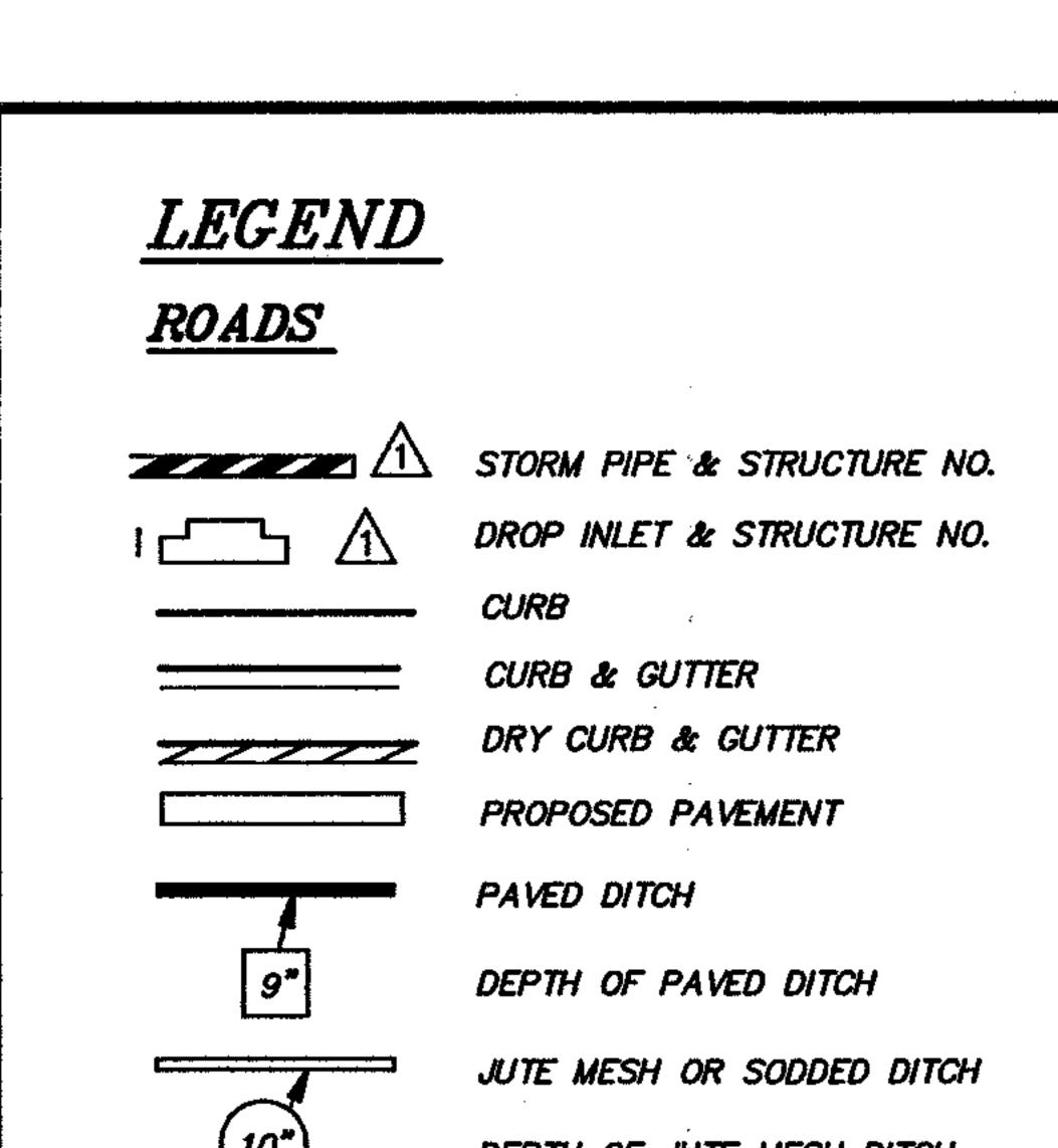
DEPTH OF JUTE MESH DITCH DRIVEWAY CULVERT AND SIZE
