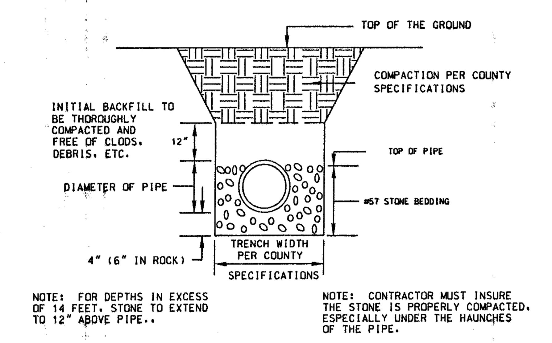
BEDDING AND BACKFILL DETAIL FOR PLASTIC SEWER PIPE
