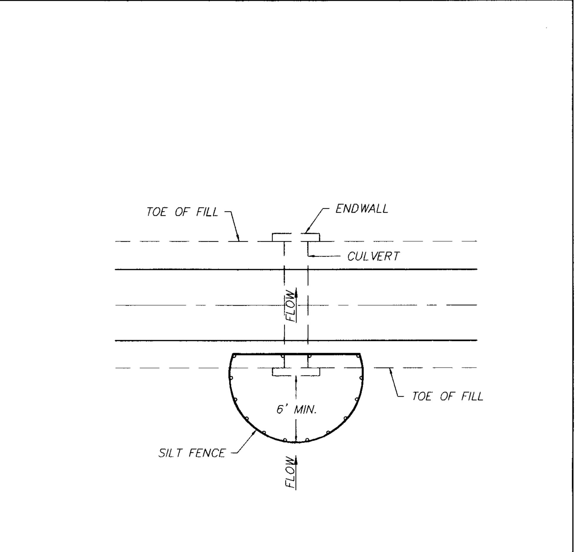
CULVERT INLET PROTECTION DETAIL
