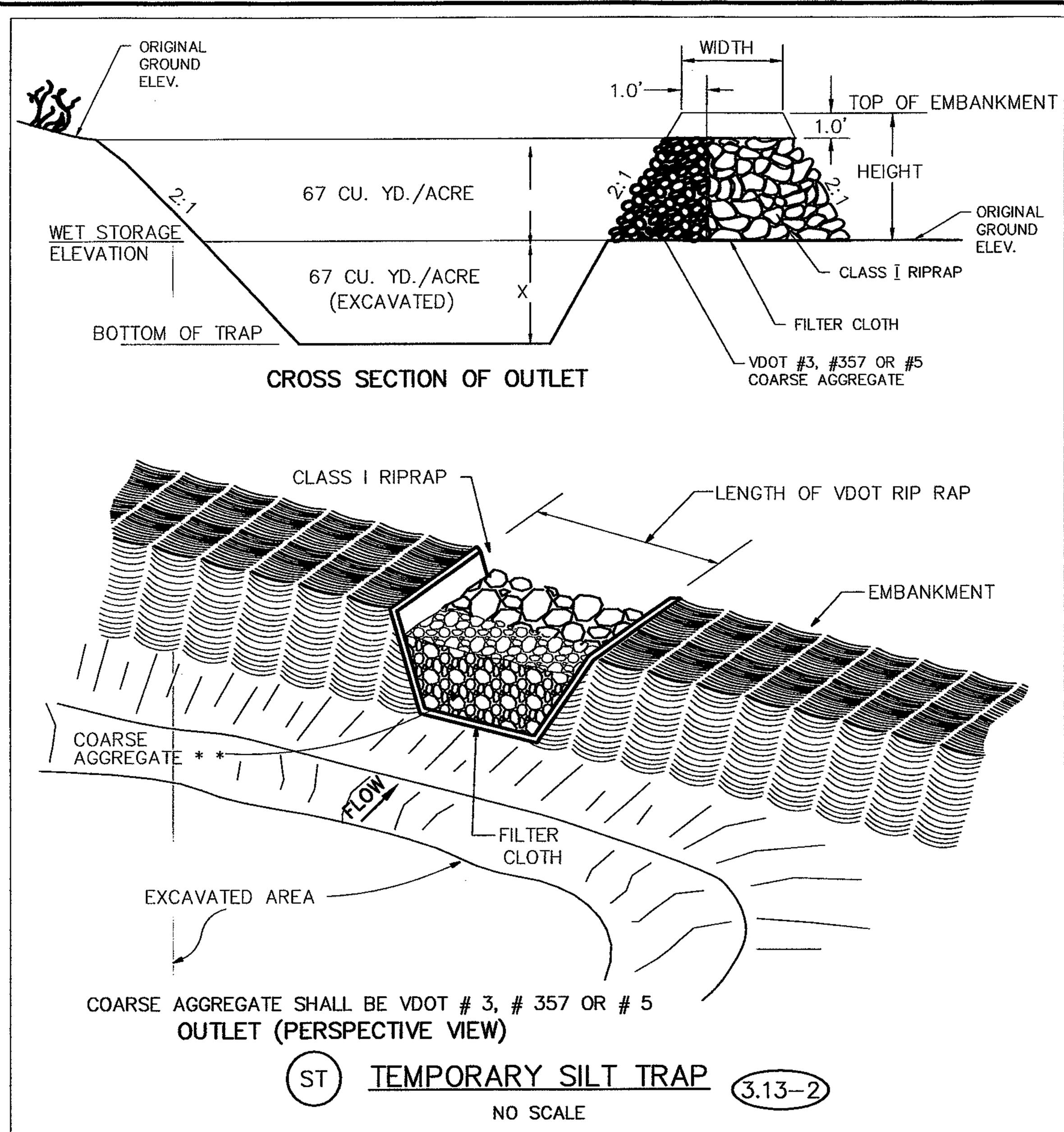
. SEDIMENT SHALL BE REMOVED AND THE TRAP RESTORED TO ITS ORIGINAL DIMENSIONS WHEN THE
